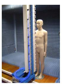
utilized for most of these areas because of its cost, size, and realtime Fig. 4 Linear antenna array. operation. However, by utilizing our high-speed radar imaging algorithm, we can offer the UWB radar as a completely new option for a variety of application fields.
