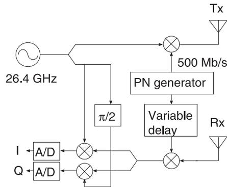
**Fig. 1.** Block diagram of the code-modulated ultra-wideband radar system.
