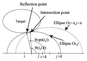
Figure 1. The principle of RPM method
