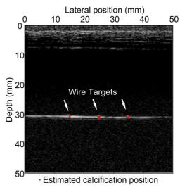
Fig. 2. Estimated wire target positions selected by the proposed method.
