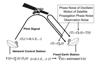
Figure 1: System model of a synchronous CDMA communication system with a GEO satellite.
