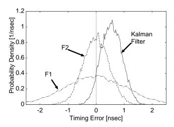
Figure 6: PDF of timing errors in three estimation methods using different filters.
