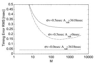
Figure 8: Relationship between RMS estimation errors and M.
