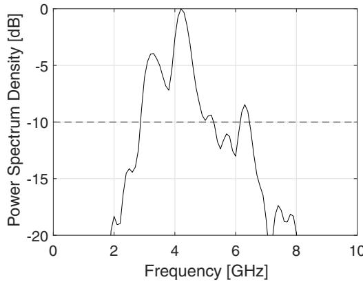
Fig. 7. Averaged power spectrum density function of the second derivative of the received signals.
