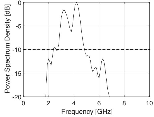
Fig. 6. Averaged power spectrum density function of the first derivative of the received signals.
