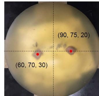
Fig. 2. Breast and cancer tissue phantom used for measurement.
