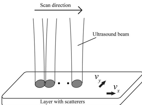
Figure 2. Simulation model used in this study.  $v_x$  and  $v_y$  are the  $x$  and  $y$  components of the tissue velocity, respectively. Ultrasound beam is scanned in the  $x$  direction.
