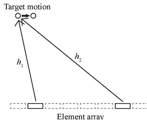
Figure 1. Target motion caused by the arrival-time difference of encoded ultrasound pulses at a measurement point.
