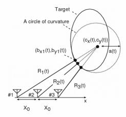
Fig. 2. Parameters of a circle of curvature.
