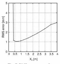
**Fig. 7.** RMS error versus the antenna distance  $X_0$
