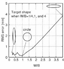
Fig. 6. RMS error versus the ratio of the long and short axis of the target.
