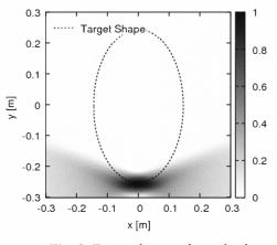
**Fig. 8.** Target shape estimated using a conventional method.
