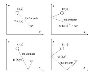
**Fig. 4**. Propagation paths between the antenna and the target via multiple reflections.
