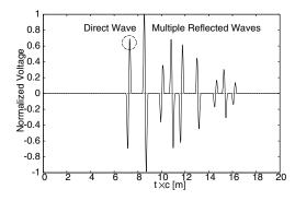
Fig. 3. An example of received signal at T = 0.
