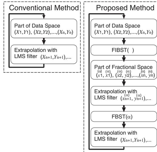
Figure 3: Procedures of the proposed and conventional quasi-wavefront extraction methods.
