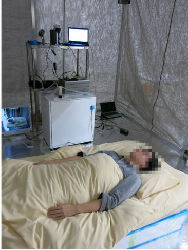
Fig. 2. Measurement setup and a participant on a bed. An infrared camera and ultrawideband MIMO array radar were installed in a cabinet. The participant had an ECG device attached to his chest.
