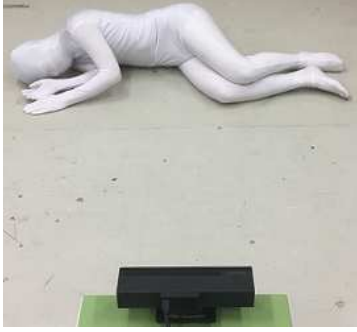
Fig. 2. Measurement setup with depth camera and participant lying on the floor.
